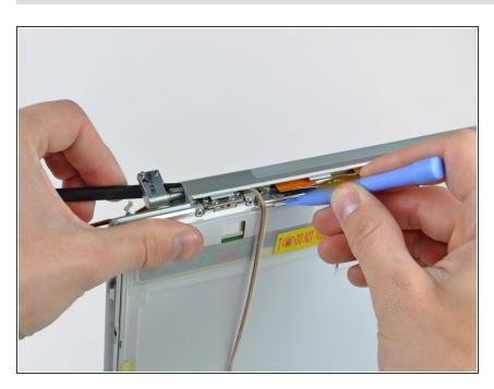
To remove the clutch assembly, first insert the flat end of a spudger into the gap between the clutch hinge
