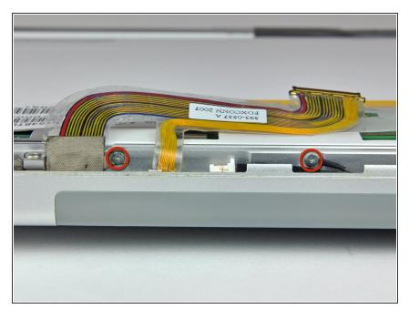
Remove the two Phillips screws securing the ground straps for the display data cable and LED driver board cable to the clutch cover.
