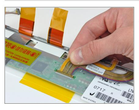
Disconnect the display data cable by pulling its connector toward the bottom edge of the display, away from the socket on the LCD.
