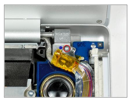
Remove the silver 9.2 mm T6 Torx securing the ground loop in the display data cable to the casing.
