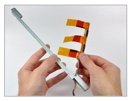
Remove the antenna cables from the clutch cover, being careful not to damage the three antenna straps.
