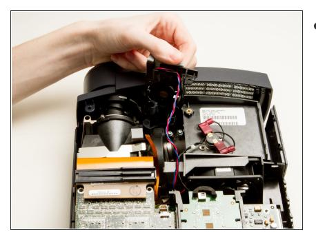
Remove the secondary fan, by pulling straight up and out of projector.
