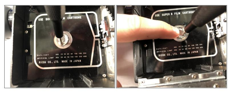
Now put your finger on the side of the screw you just removed, and take out the remaining screw with a Phillips #000 screwdriver.
