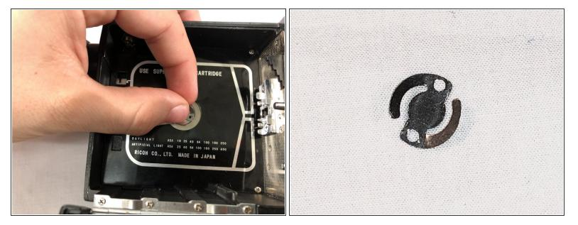
Using your fingers, gently remove the film cartridge hooks.
