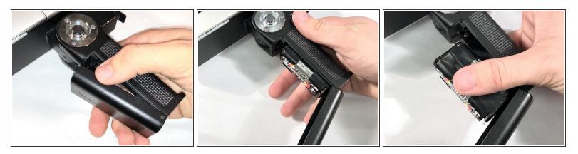
• Open the handle's battery compartment and remove the batteries from the handle.
