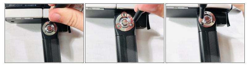
Using the Phillips #000 screwdriver, remove the three screws on the round plate on the right side of the camera handle. This is the side with the handle lock release button.
