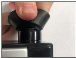
Remove the rubber covering from the eyepiece by slowly pulling down on the cover from any direction.
