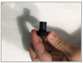
Slide the eyepiece adjuster out of the camera body.
