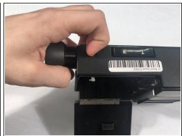
Pull the film cartridge door release lever towards the eyepiece to open the film cartridge door.
