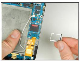
Remove the Sim Card and the Sim Card metal tray.
