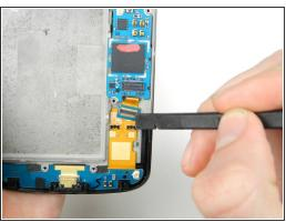
Remove the tab located in the bottom right-hand corner of the motherboard attaching the motherboard to the front display assembly using a spudger.
