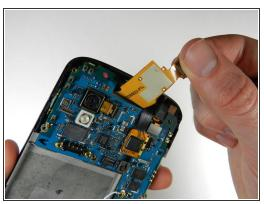
Gently pry the metal tab up using a spudger, and lift up the disconnected black flap.
