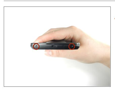
Remove the two screws from the bottom of the phone with a <u>T5 Torx</u> <u>Screwdriver</u>.
