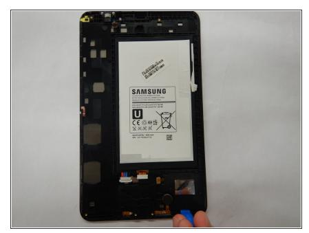
Insert the opening tool tip into the crack between the speaker and device.
