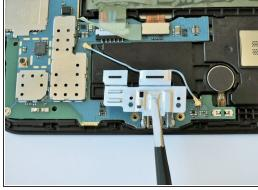
Squeeze the metal charger port cover piece with the tweezers to gently lift it from it's place.
