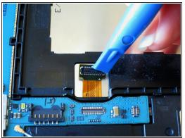
Slightly apply pressure and move the blue plastic opening tool downwards to pop the metallic rectangular connector from its socket on the mother board.
