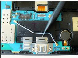
• Using the spudger gently wedge the blue wire out of its compartment.
