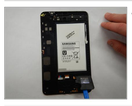
Gently pry up on the speaker to disconnect the speaker from the device.
