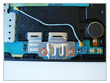
Remove two 2 mm #000 Phillips screws securing the metallic charger port cover to both the logic board and the front panel.
