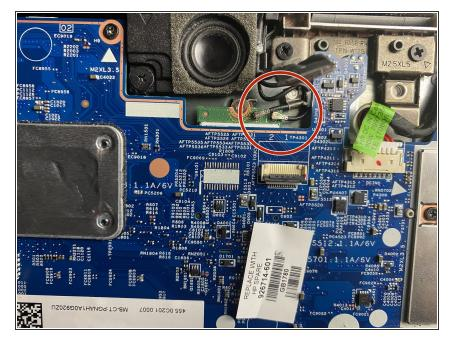
Disconnect the wires labeled 1 and 2 out.
