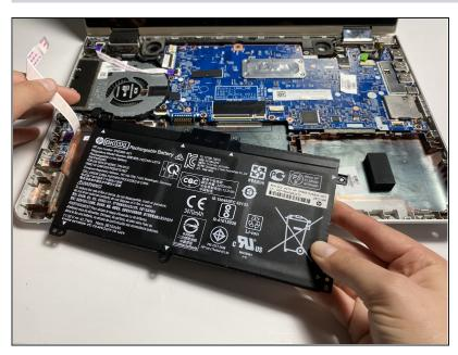
Remove the battery by gently pushing battery up, then pulling.
