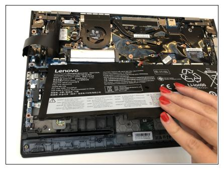
• Lift and remove the battery away from the computer.
