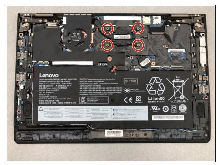
Remove four 4.5mm Phillips #1 screws from the corners of the heat sink.
