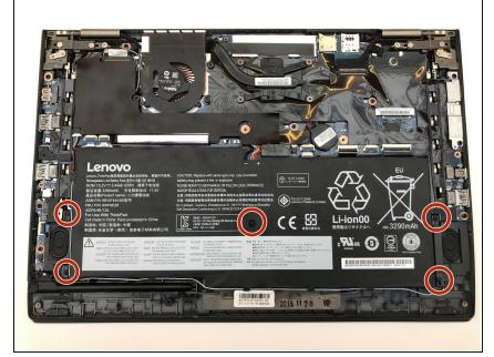
• Remove the five 4.5mm Phillips #1 screws that secure the battery.
