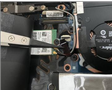
Using tweezers, pull the plastic strip out.
