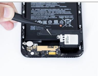
Remove the loud speaker. There are three 2.4mm Phillips #0 screws you need to remove, and one (upper right) is underneath the Xiaomi water sticker.
