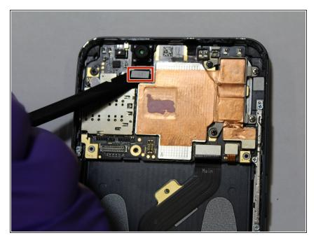
Using a plastic spudger, gently separate the front camera ribbon cable from the motherboard.
