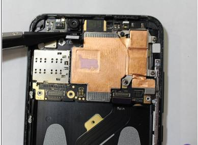
Gently use the plastic tip tweezers to remove the front camera from the back housing of the phone.
