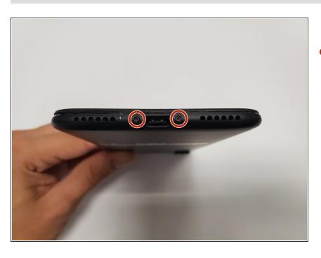
Remove the two 2.7mm Pentalobe #2 screws from the bottom of the phone.
