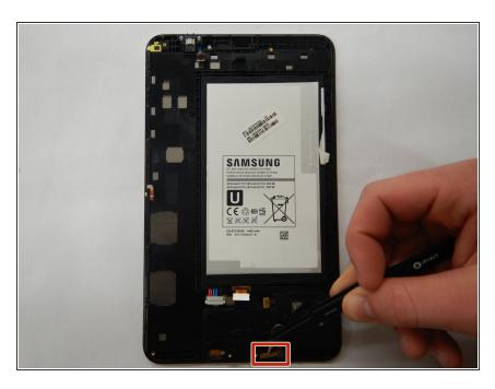
Use the angled tweezers to lift up the orange rectangular electrical connector, this will disconnect the
