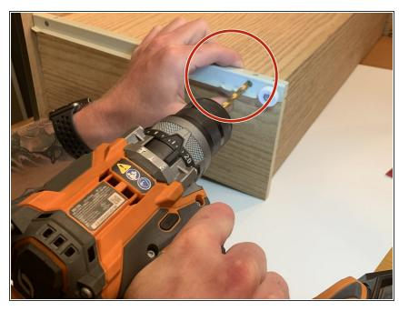
When removing rivets with a drill, wear eye protection and be cautious.
