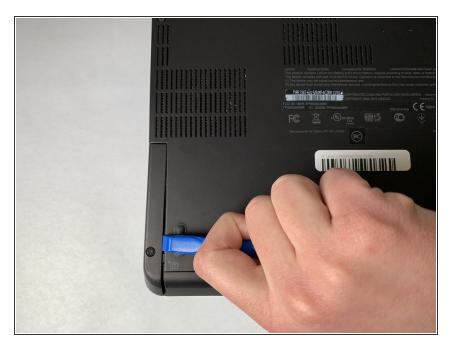
Using the iFixit Opening tool, loosen the hard drive cover.
