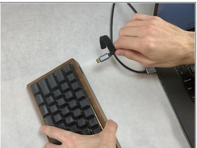
↑ Do not disassemble the keyboard or proceed with this guide if the keyboard is connected to any power source.
