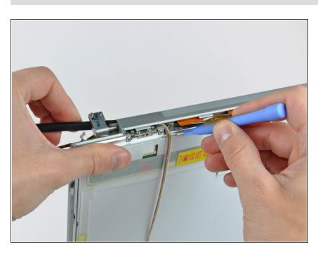
To remove the clutch assembly, first insert the flat end of a spudger into the gap between the clutch hinge
