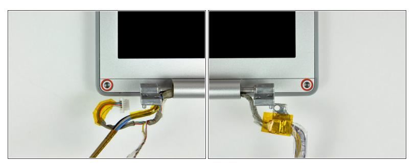
Remove the 4.5 mm Phillips screws from the lower left and right corners of the display (two screws total). These screws have a .8 mm thick head.
