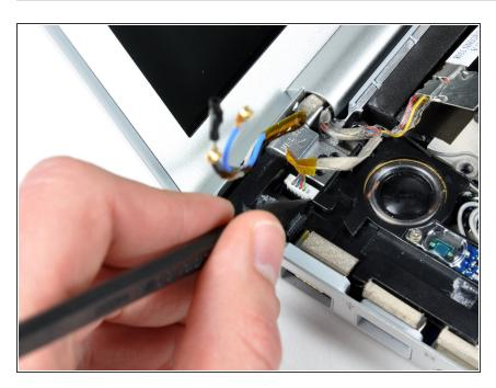
Disconnect the inverter cable from the left I/O board by placing a spudger beneath the cable and lifting up.
