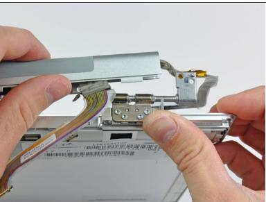
Push the clutch assembly off each of the clutch hinges and remove it from the display.
