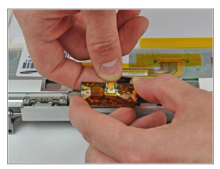
Disconnect the backlight cable by pulling its connector away from the socket on the LED driver board.
