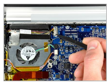
Disconnect the iSight cable from the logic board by sliding the cable to the left and out of its connector.
