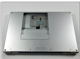
Use your fingers to push both battery release tabs away from the battery, and lift the battery out of the computer.
