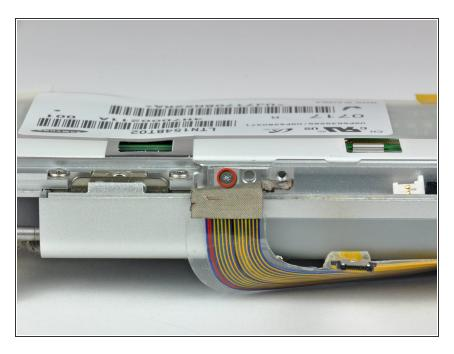
Remove the Phillips screw hidden behind the display data cable.
