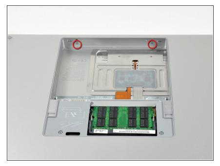
Remove the two 2.8 mm Phillips screws in the battery compartment near the latch.
