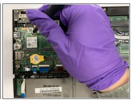
• Using a Phillips #1 screwdriver, remove the 1.3 mm screw and set it aside.
