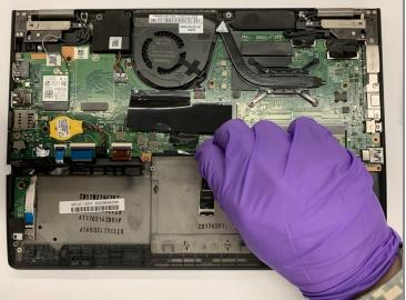
• Using your index finger and thumb gently pull the blue tab located at the top of the trackpad back from the assembly.
