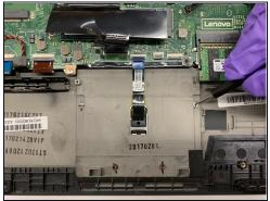
• Using a Phillips #1 screwdriver, remove the four 1.3mm Philips #1 fasteners from the back of the trackpad and set them aside.
