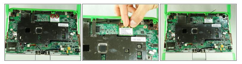
Mhen pulling out connectors, make sure to hold the metal connector instead of the wire.
