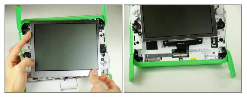
Be careful not to pull the screen out too far. There are two ribbon cables attached to the screen, and they can easily break.
