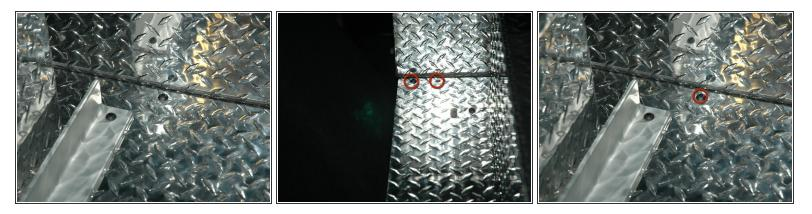
Secure plate to center support bracket with 2 bolts on the outside and on in the middle, align and finger tighten
