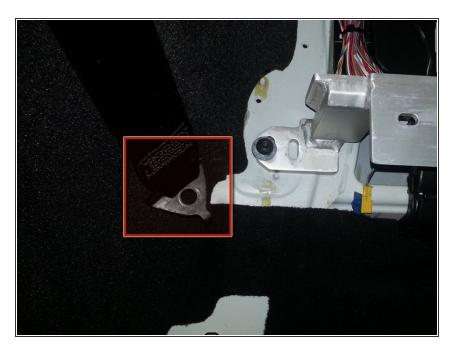
Fasten seat belt with bolt to floor
