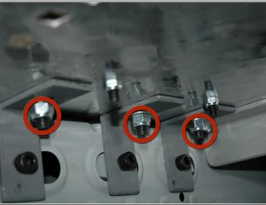
Install and loosely tighten 3 M8 black oxide bolts on each side until L bracket touches the underside of the base plate
