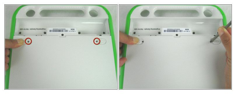
Remove the two 2mm Phillips #1 screws from beneath the battery lock tabs.
