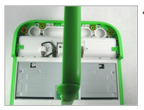
Remove the four 4mm Phillips #1 screws attaching the green trim to the body of the computer.
