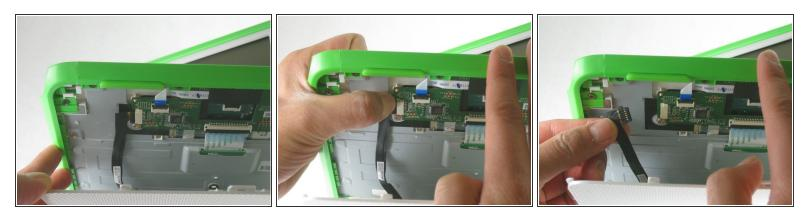
Unplug the cable from the mouse buttons controller to completely remove the lower frame from the device.
