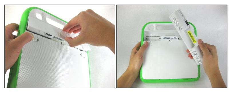
• Lift up on the middle of the battery to remove it from the device.
