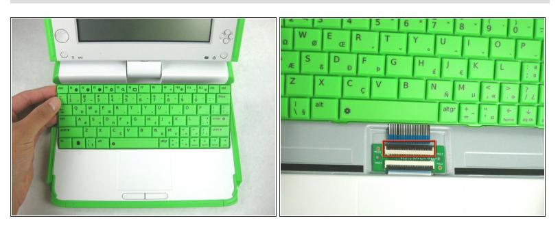
Be careful not to pull the keyboard too far because there is still a ribbon cable attached to the bottom.
