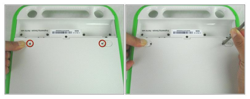
• Remove the two 2mm Phillips #1 screws from beneath the battery lock tabs.
