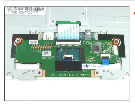
Remove the two 4mm Phillips #1 screws that attach the mouse buttons controller to the lower frame.
