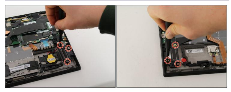
• Remove three 8mm Phillips #0 screws from both the left and right side speakers.
