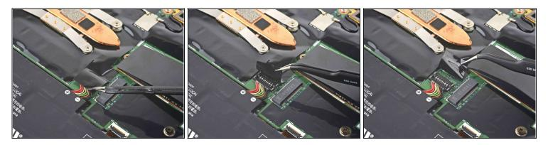
• Use <u>tweezers</u> or your fingers to peel back the plastic shield covering the battery connector.
