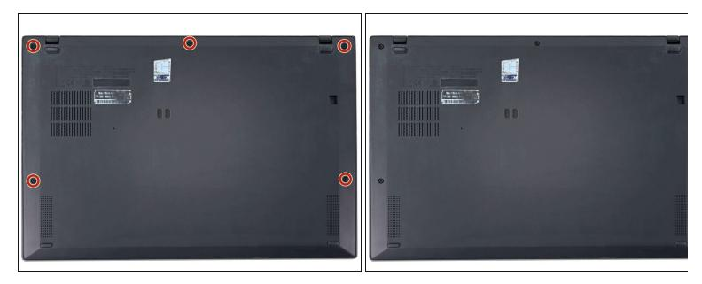
• Use a Phillips #1 screwdriver to loosen the five captive screws securing the back cover.
