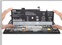
Lift the battery straight out of its recess and remove it.
