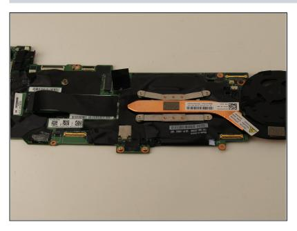
Lift the motherboard with the fan still connected straight up and out of the device.
