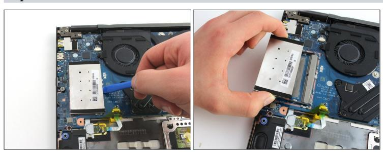
• Using a plastic opening tool or other non-metal object, pry up the large metal case on the left side of the motherboard.
