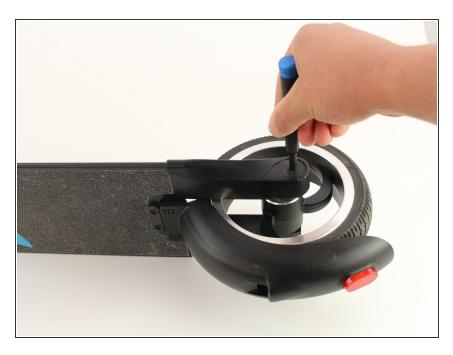
Use a Phillips #2 screwdriver to remove the 2mm screw located underneath the reflective sticker.
