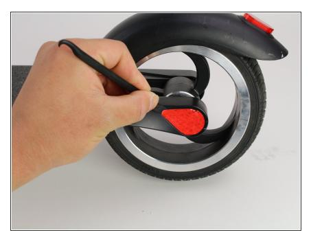
Peel off the reflective red axle sticker using a plastic spudger.
