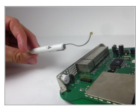
Completely separate the antenna and wire from the rest of the device.
