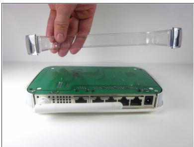
Remove the clear plastic casing by lifting it straight up from the router.
