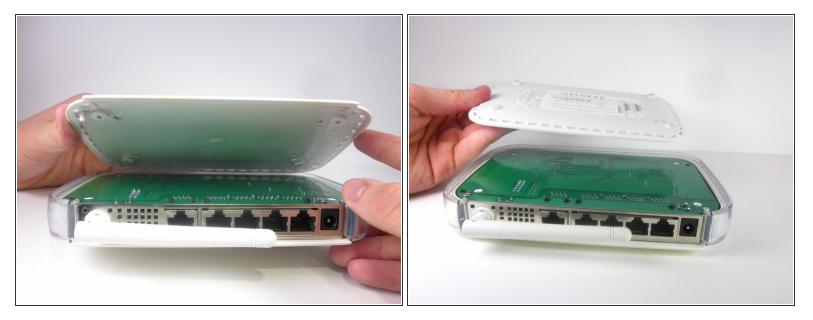
Lift the lower case straight up from the rest of the router.
