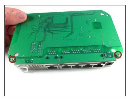
Unscrew the two 5 mm Phillips Head screws located at the front corners of the motherboard.
