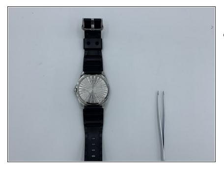
• Put the cover back and tighten it shut by pressing on it.
