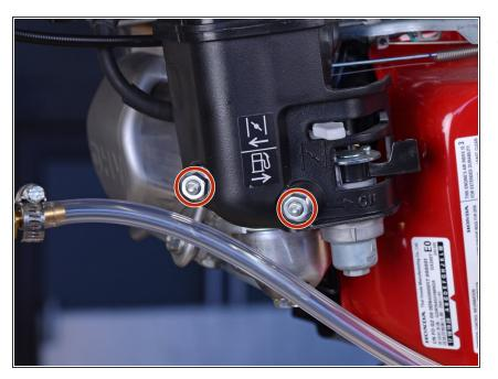
• Use a 10 mm wrench to remove the two nuts securing the air filter elbow to the carburetor's threaded rods.
