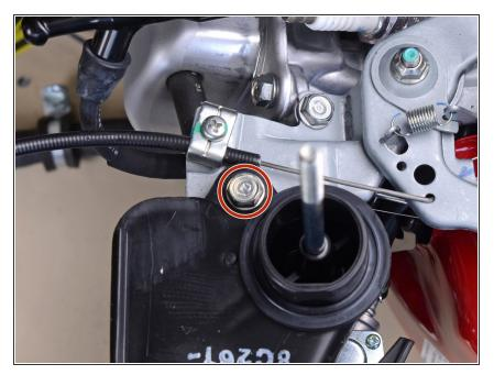
• Use a 10 mm wrench to remove the bolt securing the air filter elbow to the concrete saw.
