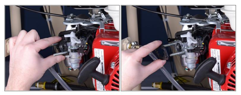
• Pull the carburetor spacer straight off, making sure it clears the threaded rods.
