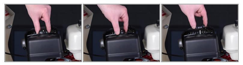
• Use your fingers to unscrew and remove the wing nut securing the air filter cover.
