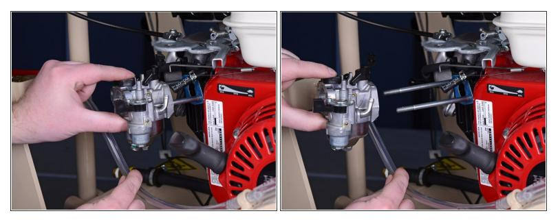
• Pull the carburetor straight off of the threaded rods to remove it.
