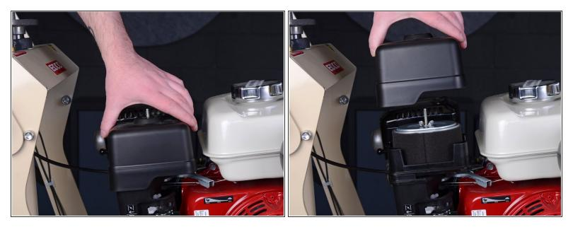
• Lift the air filter cover straight up to remove it.
