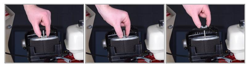
• Use your fingers to unscrew and remove the wing nut securing the air filter.
