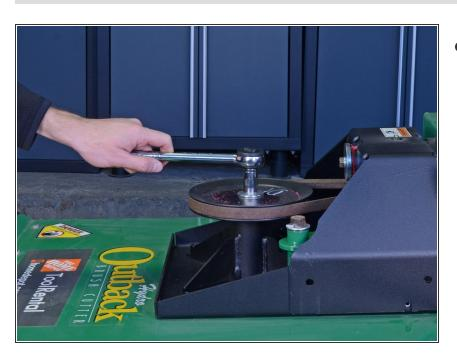
Using a 9/16" socket or wrench, make sure the bolt at the top of the spindle is tight.
