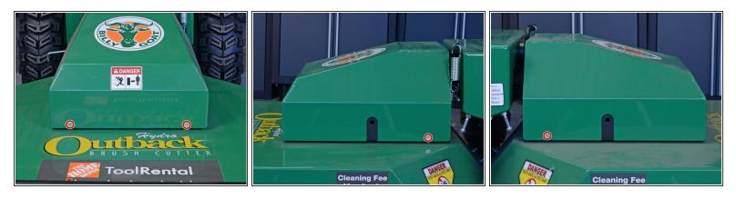
Use a 3/8" socket or wrench to remove the four 21 mm bolts securing the top cover to the deck.
