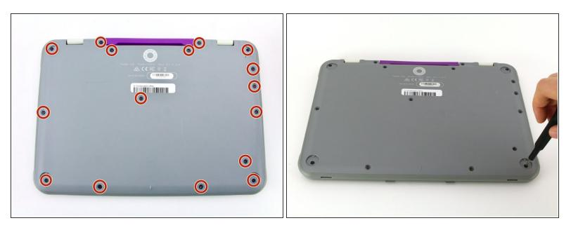
• Using a Phillips #00 screwdriver, remove the sixteen 5.0 mm black screws from the back panel.
