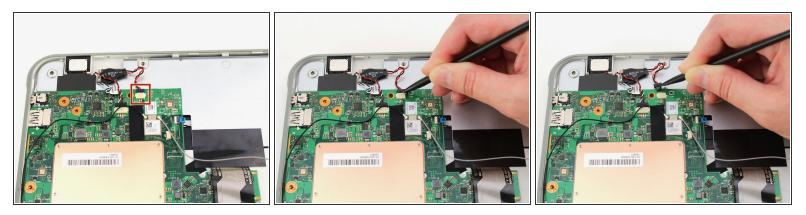
Use a plastic spudger to slide out the cable connector attached to the CMOS battery from the motherboard.
