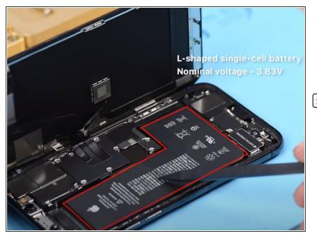
iPhone 11 Pro has a bigger battery capacity than iPhone X series. We can see clearly that the battery is a little thicker.
