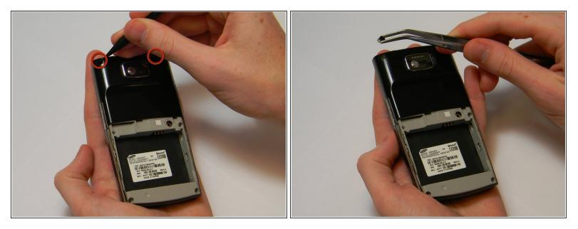
Use the spudger to pry the two plastic caps out of the top corners of the phone casing.
