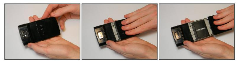
• Apply downward pressure to the top of the battery panel while pulling down to slide it off the phone.
