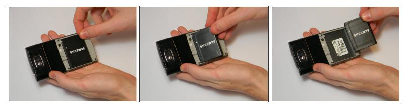
• Locate the grooves on the sides of the battery near the bottom of the phone. Use your fingers to pull the battery up and out of the phone.
