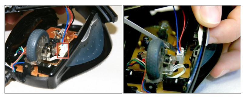
Use a spudger to pry underneath the white plug and pop it out to disconnect the upper board from the lower board.
