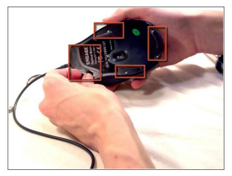
Flip the mouse over and peel off the stickers on the perimeter of the bottom of the mouse.
