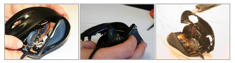
• Grab the top shell of the mouse and lift up to remove.
