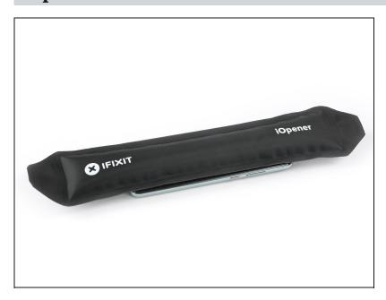
Apply a <u>heated iOpener</u> to the screen and all edges of the phone to loosen the adhesive beneath the edges of the LCD screen and digitizer. Apply the iOpener for at least two minutes.
