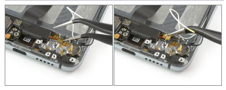
• Use one arm of a pair of tweezers to peel up the contact cable of the loudspeaker.
