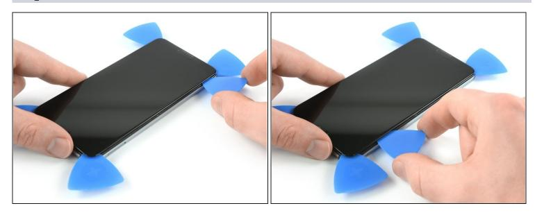
• Insert a fifth opening pick and slide it along the left edge of the phone to cut the remaining adhesive.
