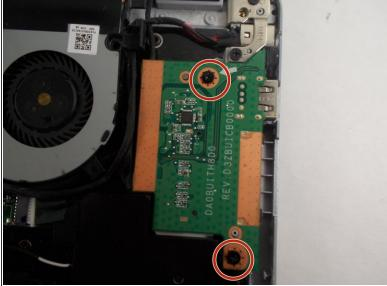
Remove the screws attached to the USB board.
