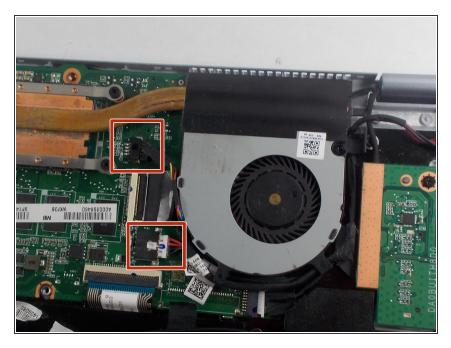
Detach the wires connecting the fan to the motherboard.
