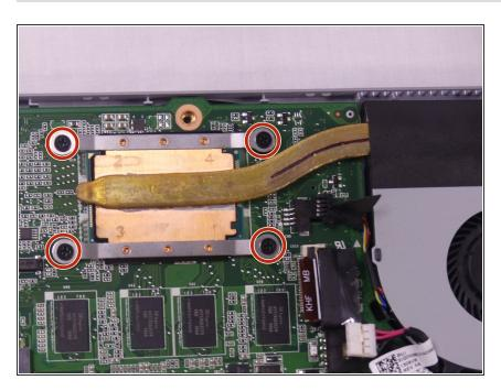
Unscrew the four captive Phillips #0 screws from the heat sink.
