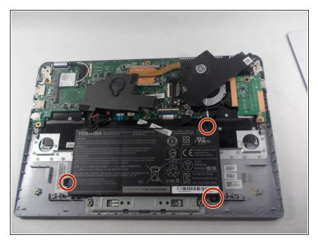
Remove the three Phillips #0 screws from the battery.
