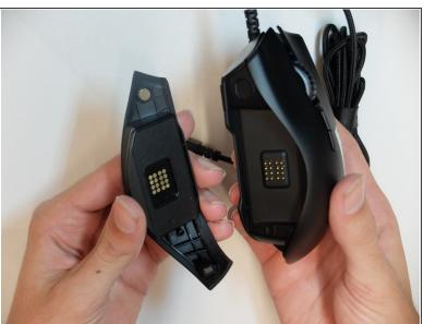
Remove the interchangeable side plate.
