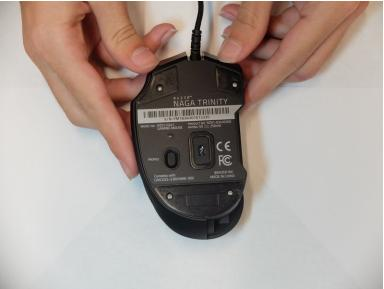
Remove the mouse's feet using the opening pick.
