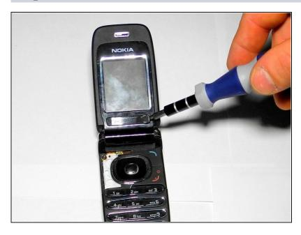
Using a <u>2.0 flathead</u> screwdriver, pry open and remove the black, plastic strip (beneath the screen) to reveal the 2 screws holding the screen in place.
