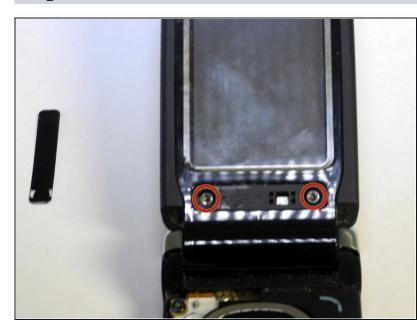
Remove the two T6 Torx screws from the base of the display.
