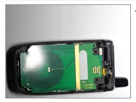
• To reassemble your phone, reattach the display to the phone by reconnecting the display ribbon cable. Place the screen assembly back into the front case of the phone.
