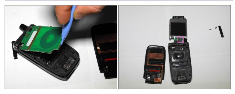
• Use a plastic opening tool to pry the LCD circuit board up and out of the phone.
