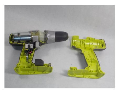
Lift and remove the casing off of the drill body.
