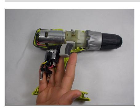
Carefully lift and remove the battery clip, trigger, motor, and everything connected to the wires and pull straight out of the drill.
