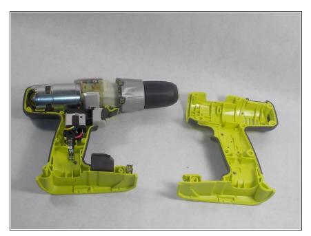
Using your hands, lift and remove the right cover of the drill body off from the left side and place it down.
