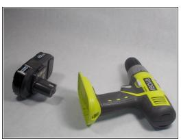
Detach the battery unit from the drill body by pressing the battery release buttons on both sides of the unit and pulling outwards.
