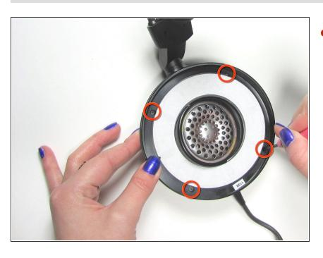
Remove all four 1cm screws on the inside of the headphone using a #1 Phillips head.
