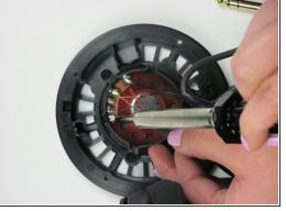
Re-solder the new red, yellow, and blue wires using a soldering iron. If you need assistance, reference <u>How To Solder and Desolder Connections</u>.
