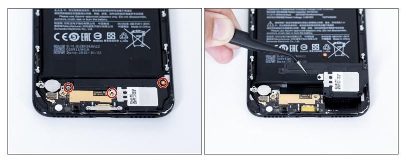
Remove the loud speaker. There are three 2.4mm Phillips #0 screws you need to remove, and one (upper right) is underneath the Xiaomi water sticker.
