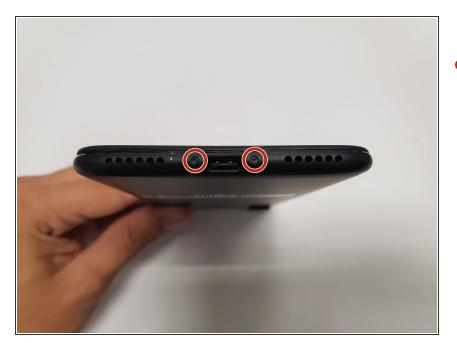
Remove the two 2.7mm Pentalobe #2 screws from the bottom of the phone.
