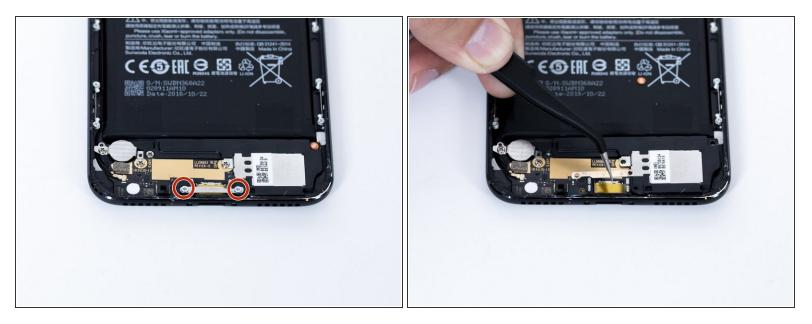
• Remove the two 3.8mm Phillips #0 screws holding down the lower metal bracket.
