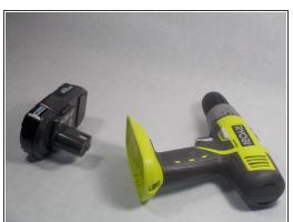
Detach the battery unit from the drill body by pressing the battery release buttons on both sides of the unit and pulling outwards.
