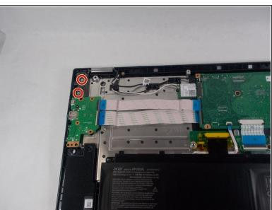
Remove the five 6mm Phillips #1 screws from the hinges on either side of the laptop.
