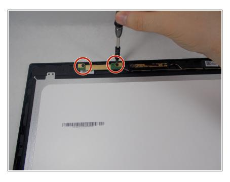
Remove the two 3 mm Phillips #1 black screws from the microphone at the top of the display cover.
