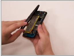
Use an opening tool or fingers to separate the midframe covering the rest of the device starting at the top corner.
