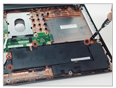
• Using the Phillips #000, remove the four 9.5mm screws around the battery.
