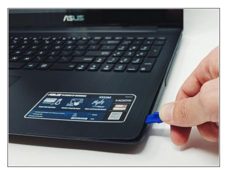
• Using the iFixit Opening Tool, pry the keyboard off.
