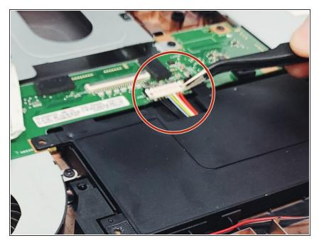
• Carefully disconnect the battery's 8pin connection to the motherboard.
