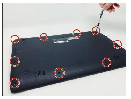
• Turn the laptop over. Using the Phillips Head 000 bit, remove the four 4.8mm screws from the bottom edge. Use the same bit to then remove the remaining six 9.5mm screws.
