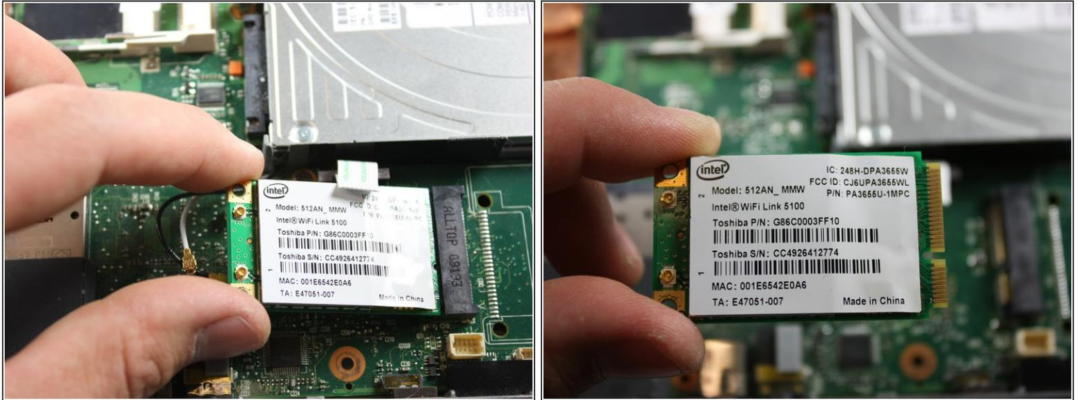
**⚠ Be careful not to pull the WiFi card straight up, as you might damage components on the motherboard.**
